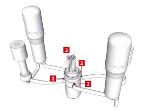
Vital points in the primary circuit are being monitored by **thermocouples** [2] since 2010. They record any load changes as a result of changes in temperature. The data can be used to draw 'real-time' conclusions about fatigue in the primary circuit.
