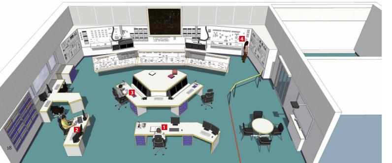
A special panel allows the deputy shift supervisor to monitor the nuclear plant's critical safety functions, including conditions in the primary system, the functionality of the containment structure and conditions in the reactor.
